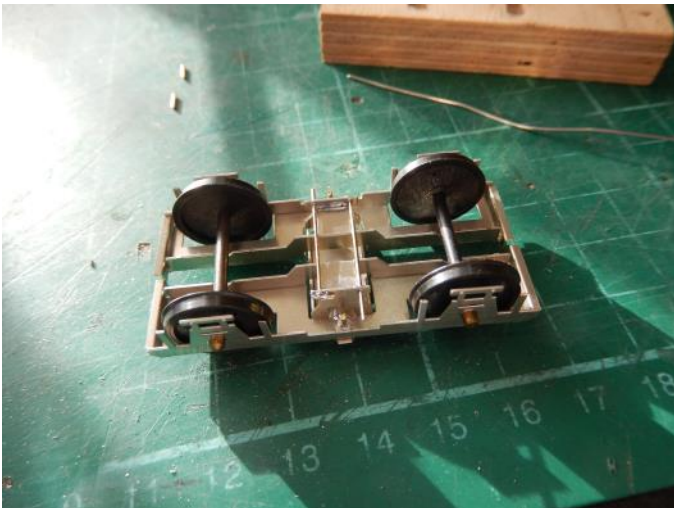
Wheels put in place after the inner rivets have been shortened so that the bogie can be turned over. Torsion bars are soldered to the brackets gently squeezing both sideframes together so there is little or no sideplay in the wheel bearings.
