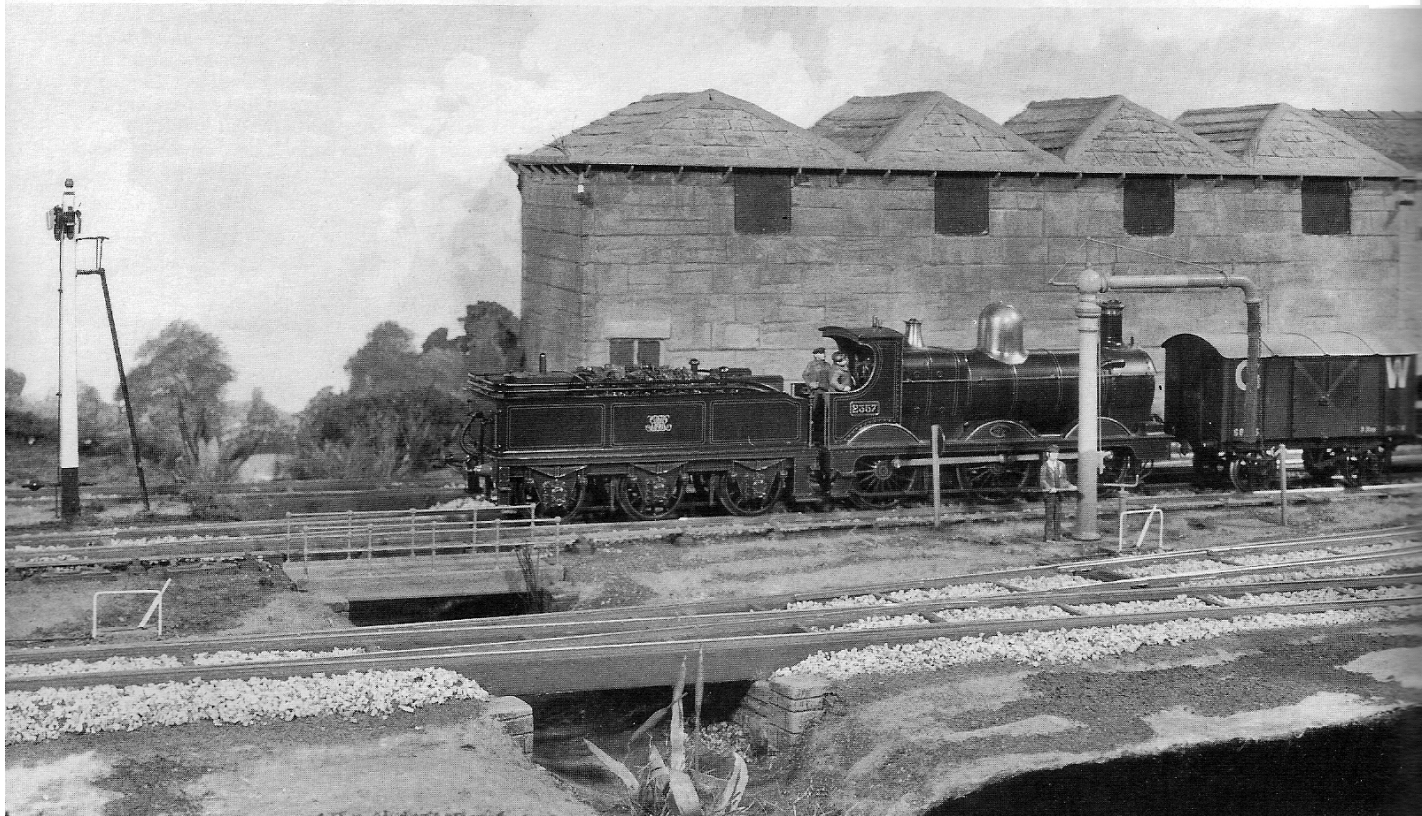
Like all the author's locos, Dean Goods No. 2357 is powered by a Portescap RG7 motor and features a fully-sprung split-framed chassis.
