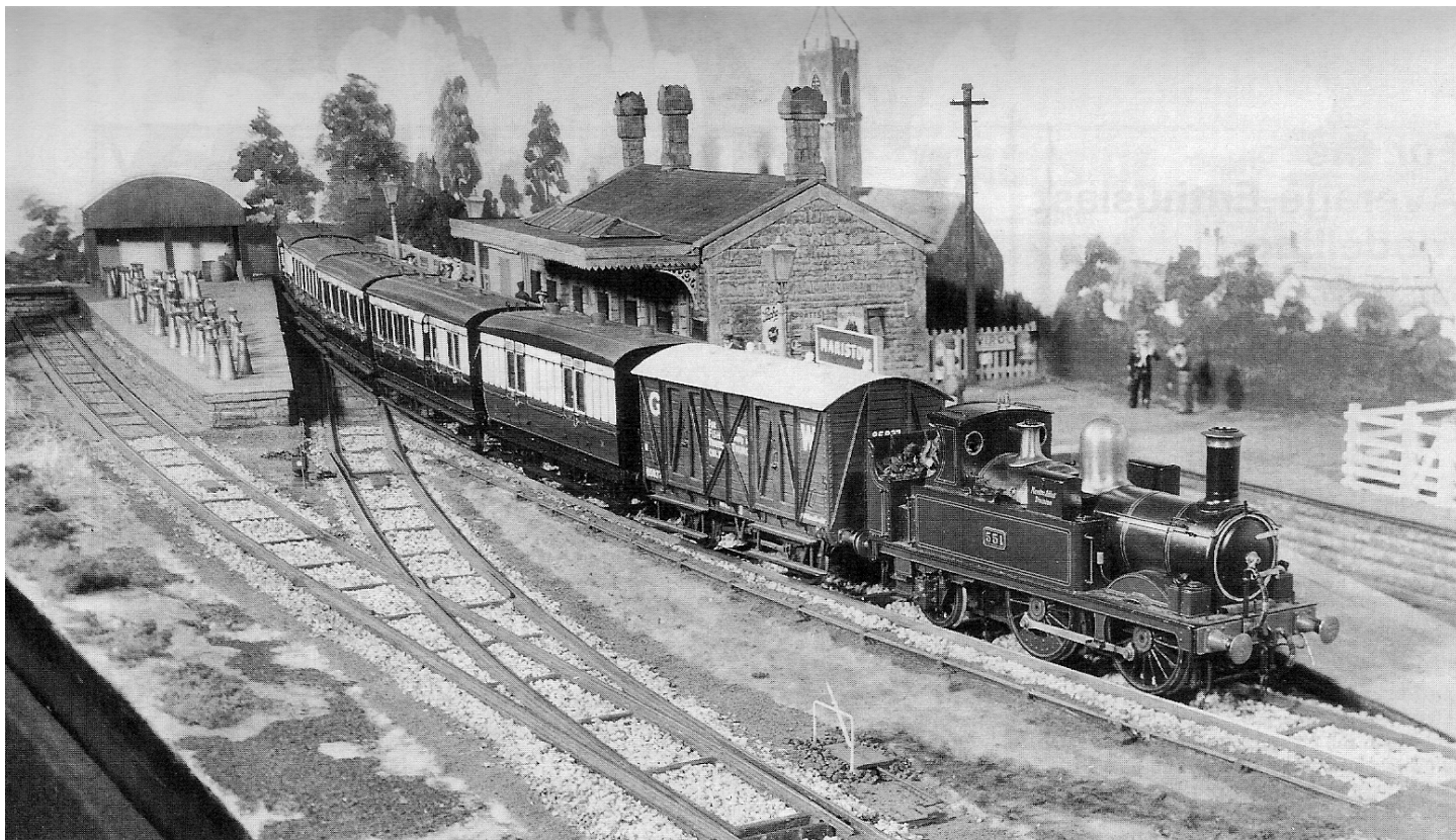
Morning passenger train ready to depart for Plymouth, composed entirely of 4-wheeled stock and headed by 517 Class 0-4-2T No. 551, painted in the pre-1906 livery with Indian Red frames.
