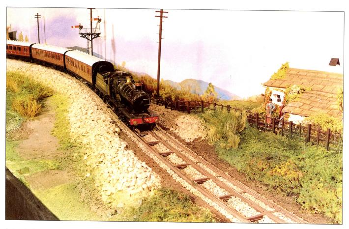
look at (and even worse to build!), but as this area is all constructed with rail soldered to copperclad sleepers, it was much easier than it would have been if prototypical appearance had also been important.
