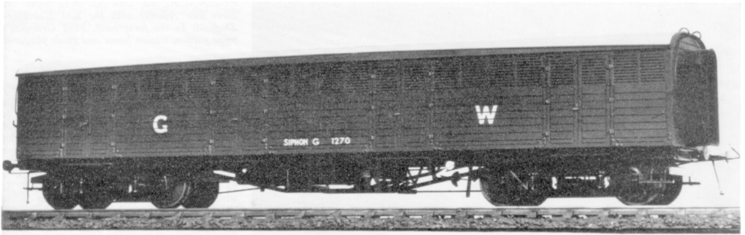
3 Outside framed 50ft. Siphon G.
