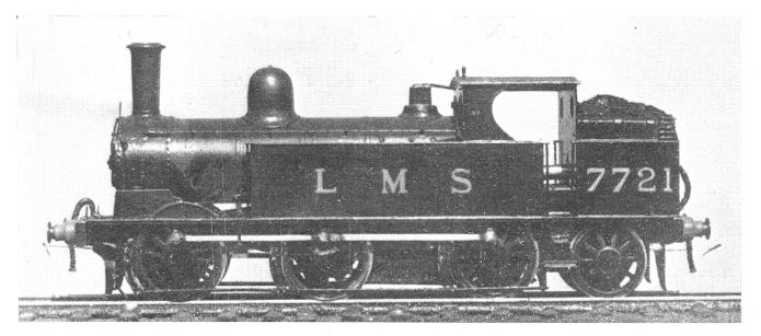
a wheel base point of view the locomotive is arranged like an 8-coupled one. It will traverse a curve of 2 ft. 6 in., with side play of 0.010 in. in the middle axles, but in practice the minimum curves are 4 ft.
