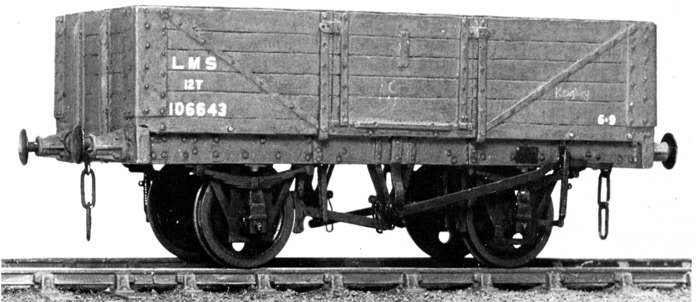
This LMS Diagram 1666 wagon is scratchbuilt. I experimented with sprung buffers on this one, and the right-hand buffer appears to be pushed in. Amazingly, the model has sagged at the ends in exactly the same way as the prototype and to just the right degree! Check by placing a ruler along the lower edge of the solebar. Note also properly joggled V-irons. The LMS had 70 of these wagons for each 4F!
