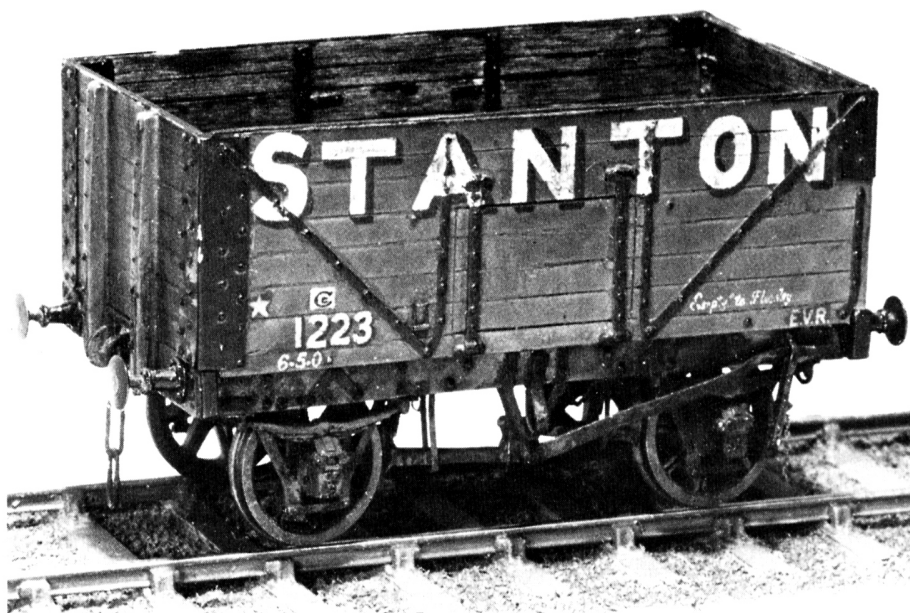
The prototype of the Stanton wagon was built by Eastwoods. 1223 started life with side, bottom and end doors, but the end door was blanked off and the small corner plates fitted, probably in pre-grouping days. The letters EEC (Edward Eastwood, Chesterfield) are reproduced on the scratchbuilt Ellis axleboxes. We now think of Stanton as ironworks, but in pre-nationalisation days they were also colliery owners in quite a big way.
