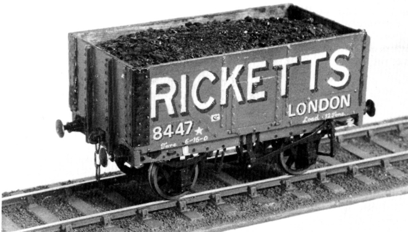
This wagon was built early in 1974 from a picture in the Model Railway Constructor. I suspect now that a post-war photograph was used to prepare the illustration – the tare weight seems very low. I have chosen this photograph to illustrate the too thin lettering – a common error among beginners – and the incorrect hanging of the brake safety loops. I didn't know about middle bearers when I built this one!
