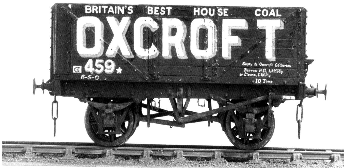
The Oxcroft wagon. I have selected this shot to show the nuts on the ends and the bottom door pins and chains. This model was built in 1978 to a sketch by Gordon Heywood. The prototype really did have unevenly-spaced lettering, apparently. Note the lack of a black line between the letters and the shading – I hadn't learnt this trick in 1978!
