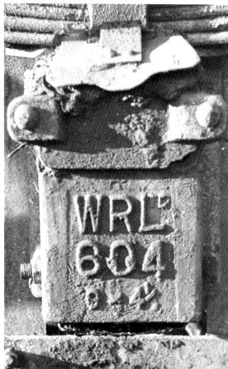
Left: An Ellis patent axlebox with 9 in x 4 1/4 in journals fitted to a 12 ton wagon by Wagon Repairs Ltd. Main dimensions are: Across front face 8 in. Axleguard front to face of box 9 in. Bottom of box to bottom of lid 11 in. Bottom of box to spring bed 11 7/8 in. Right: A Rigley's patent axlebox under a preserved 10 ton wagon. Main dimensions are: Across front face (bottom part of box) 6 7/8 in. Axleguard front to face of box (bottom part) 9 in. Depth of bottom of box 3 5/8 in. Depth of top of box (to bottom edge of lid) 6 1/8 in. Depth of lug on right 2 5/8 in. Projection of lug from side of box 1 1/8 in. AUTHOR
