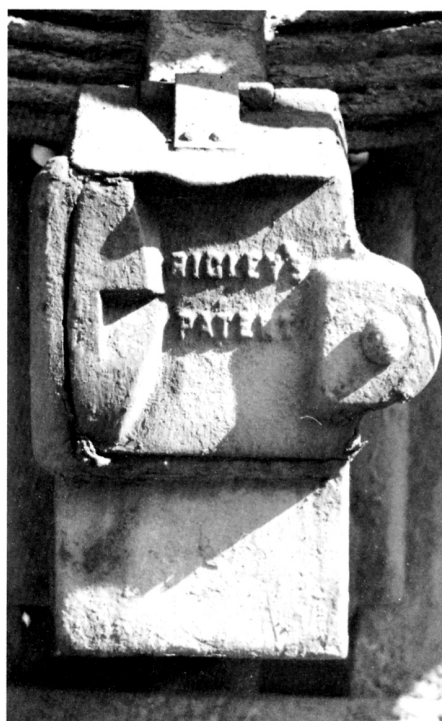
Left: An Ellis patent axlebox with 9 in x 4 1/4 in journals fitted to a 12 ton wagon by Wagon Repairs Ltd. Main dimensions are: Across front face 8 in. Axleguard front to face of box 9 in. Bottom of box to bottom of lid 11 in. Bottom of box to spring bed 11 7/8 in. Right: A Rigley's patent axlebox under a preserved 10 ton wagon. Main dimensions are: Across front face (bottom part of box) 6 7/8 in. Axleguard front to face of box (bottom part) 9 in. Depth of bottom of box 3 5/8 in. Depth of top of box (to bottom edge of lid) 6 1/8 in. Depth of lug on right 2 5/8 in. Projection of lug from side of box 1 1/8 in. AUTHOR
