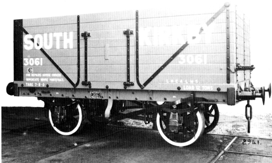
This wagon, from the same builder, looks identical in construction to the Thorne wagon. However, in this case the side knee washer plates are bent round at the bottom, and there are small brackets between the side rail and the solebar, taking the inner, lower washer plate bolts. On the original prints it is possible to see that the brake levers are different, that on the South Kirkley wagon having simply a bent end instead of a loop. It is small differences like these that make the study and modelling of wagons so fascinating.
