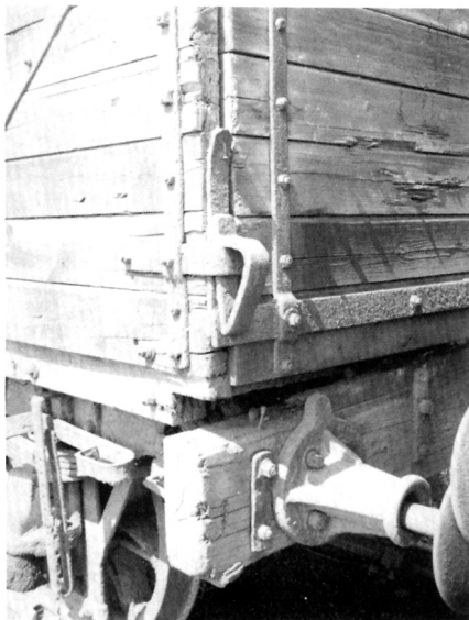
D-dropper end door fastener – very fiddly to model! Note also round-based ribbed buffer, with lip to keep door sill in, single strapbolt washer plate and flat piece of iron bolted to headstock, also to keep door sill in.
