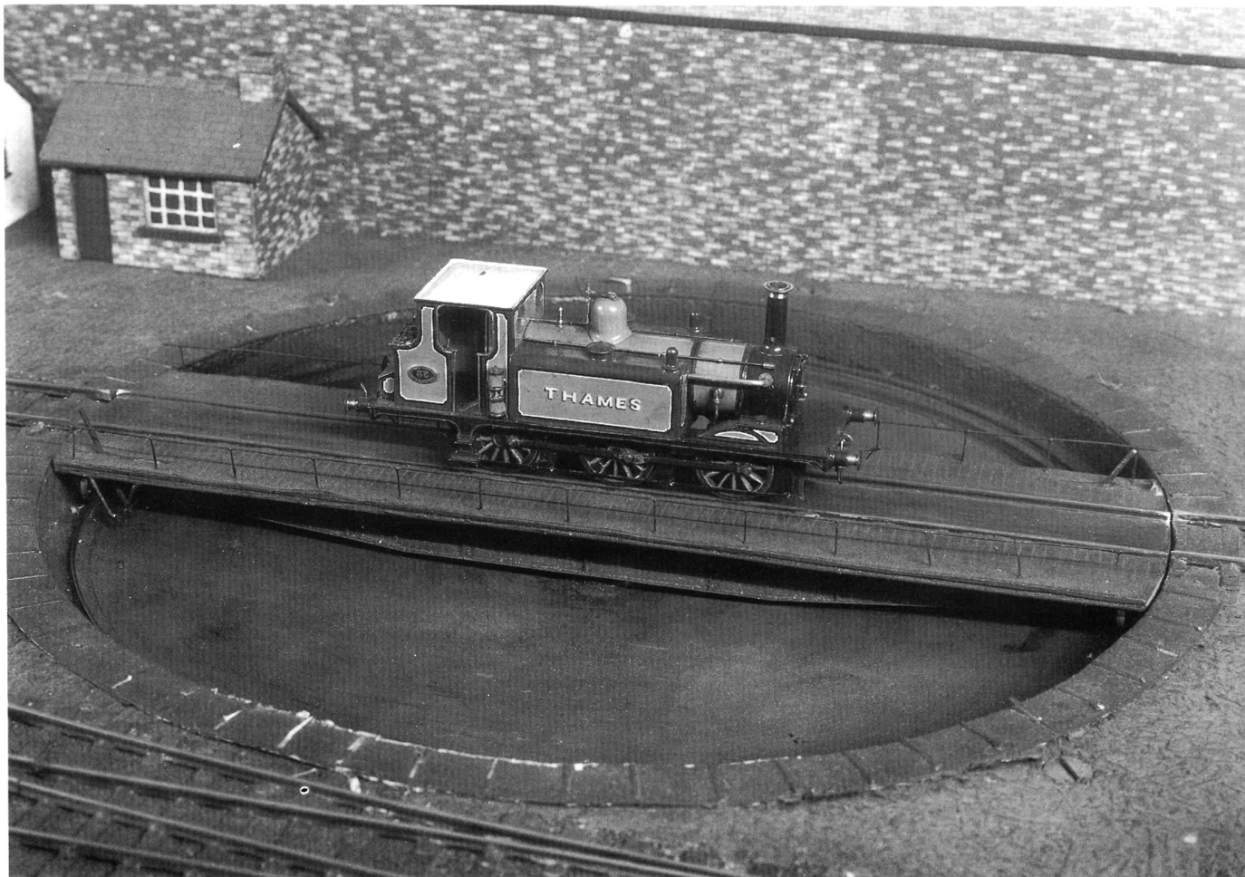
The Terrier, dwarfed in the centre of the bridge, shows that this is the sort of large-diameter turntable that can cope with anything. But with sub-surface tables, the bigger they are, the harder they are to model. This is Sid Stubbs's 80ft Cowans Sheldon table -- exactly the same as the one described by Norman Dale here. The signs of wear can be explained by the fact that Sid built this in 1951!
