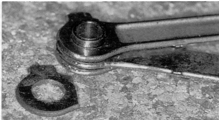
Left: Components of the connecting rod big end. The phosphor-bronze bush helps to locate everything. Right: Soldering components held together with clips and an old broach.
