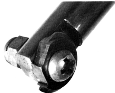
The circular form tool for machining the worm and the hob.
