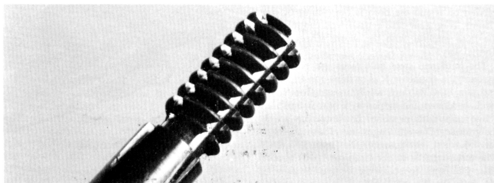
The hob. It can be sharpened with one of those thin slitting/grinding wheels used in small power hand-drills.
