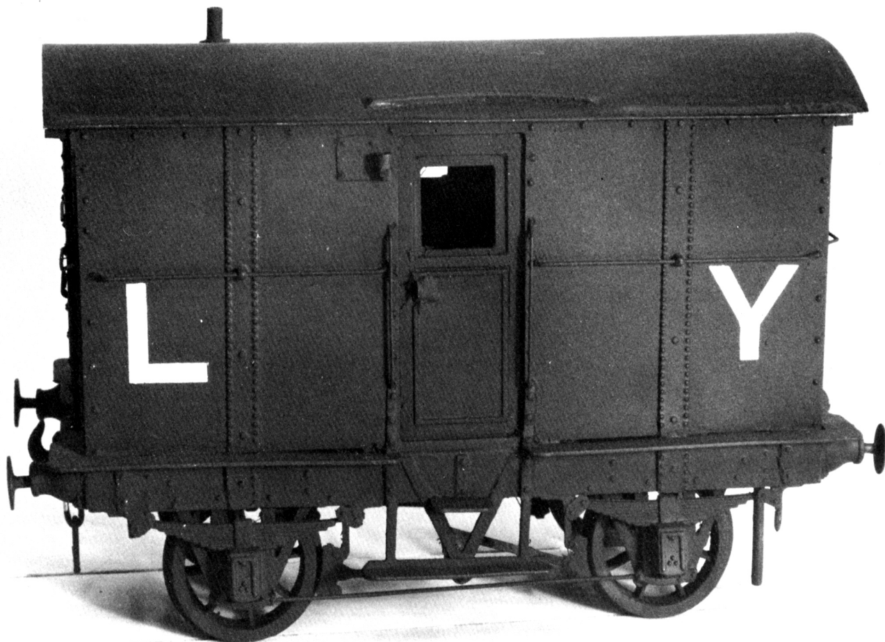
The kit brake van built up as supplied. The side lamp position is in the wrong place and should be on the right-hand side of the door which is hinged wrongly too. I have positioned the rainstrip correctly and the lamp iron was moved after this photograph had been taken. The author's scratchbuilt model of one of these vehicles was illustrated in MRJ No. 2.
