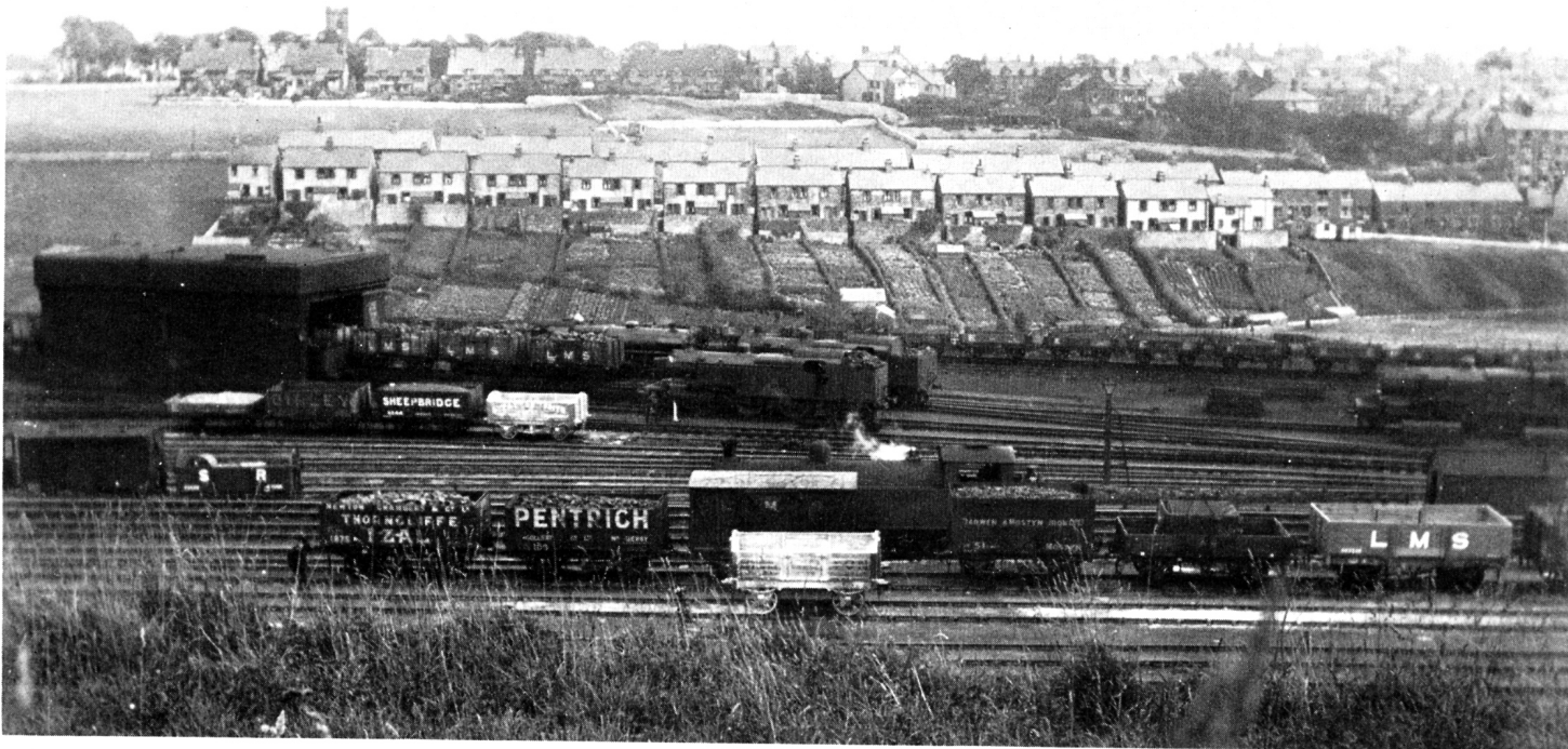
A scene at Buxton c.1934. The Birley, Sheepbridge and Thorncliffe wagons must have travelled via Dore and Chinley. The Pentrich wagon would arrive via Ambergate and Millers Dale. S. Taylor, Frith and Bibbington are local lime wagons. The presence of a Darwen & Mostyn Iron Co. Ltd. wagon is interesting. LMS wagon 403325 (last digit not clear) is a rare example of a wagon to Diagram 1896 photographed in service. Note that the Thorncliffe wagon is carrying coal – not Izal!
