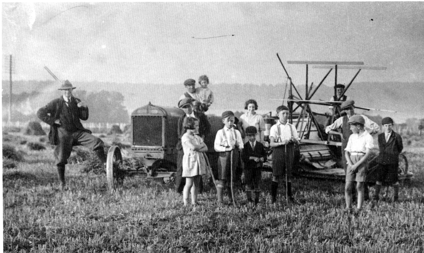
An 'International' 10/20 tractor and binder. Two men were required to work this tackle; cutting with scythes would have clearly required many more. One of the children is my father. COLLECTION TIM WATSON
