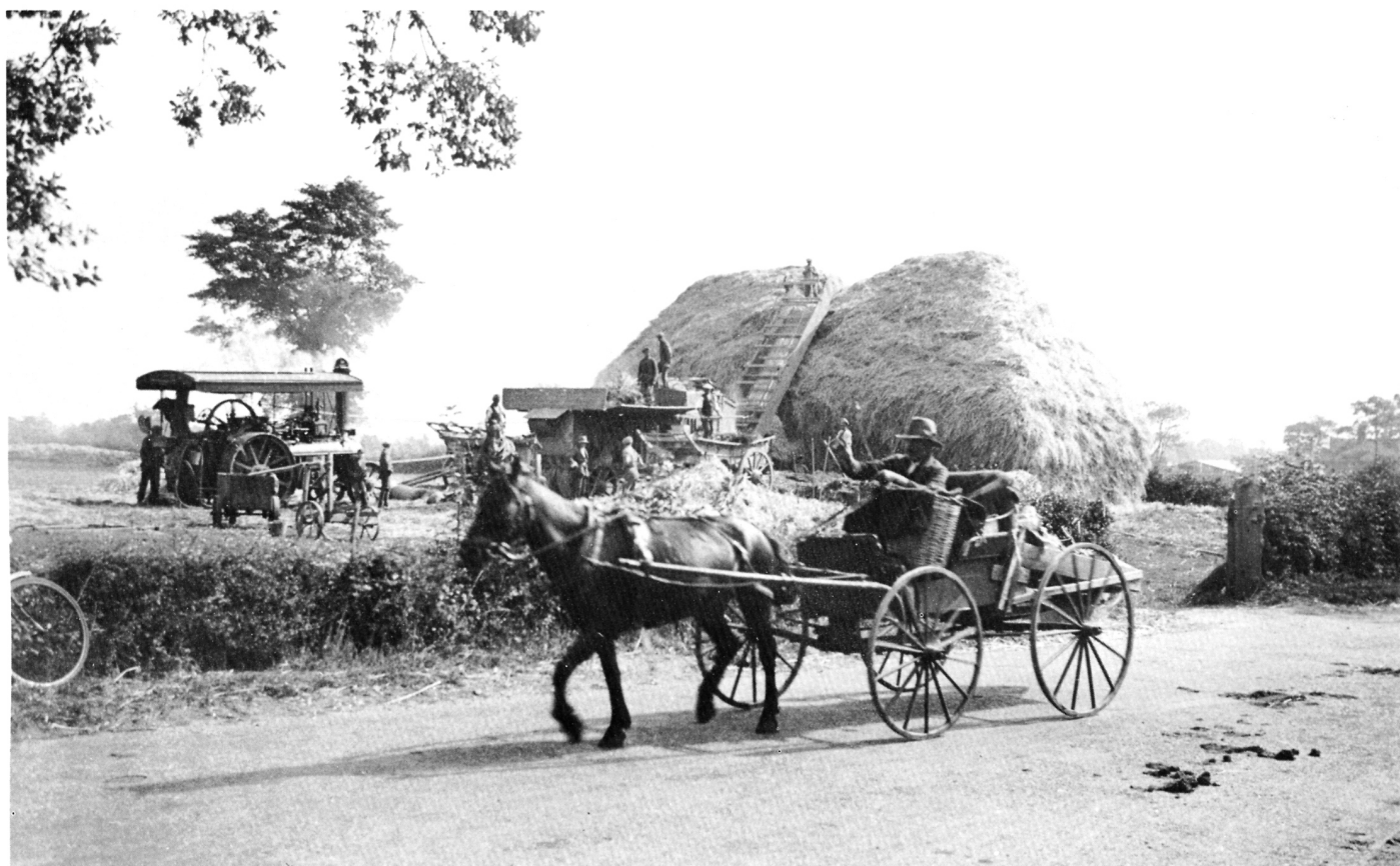
Over the hedge at Laxfield, Suffolk, in 1935, a canopied traction engine drives a threshing drum (centre), while an elevator raises the stack of 'threshed' straw – probably driven by the horse gear visible in front of the locomotive. The original unthreshed stack has all but disappeared. A good modelling point is the fineness of the wheels on the little pony cart in the foreground. S. H. FREESE
