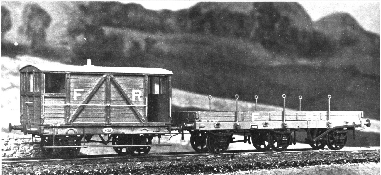
Models of the standard 10ton goods brake van and a 6-wheeled plate wagon.
