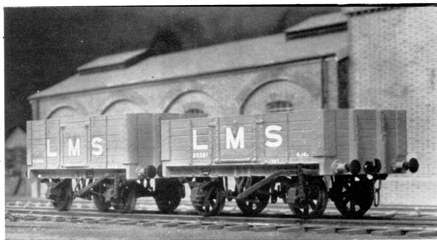
Heading photo: Ex-MR dropside wagon 13615. Ex-LNWR open wagon 225139. The shape of the brake levers betrays the origin of these wagons as also the headstocks of 225139. I hope there will soon be castings available for the distinctive lop sided LNWR Buffers. Above: Ex-MR wagons 95868 and 20261. This is the later Midland design. Buffers are ABS LSWR-type (just right for the MR). Axleguards are K's and brake gear Kenline 10ft wheelbase shortened to suit the 9ft 6ins wheelbase. Notice how the Midland did not always use very short brake levers.
