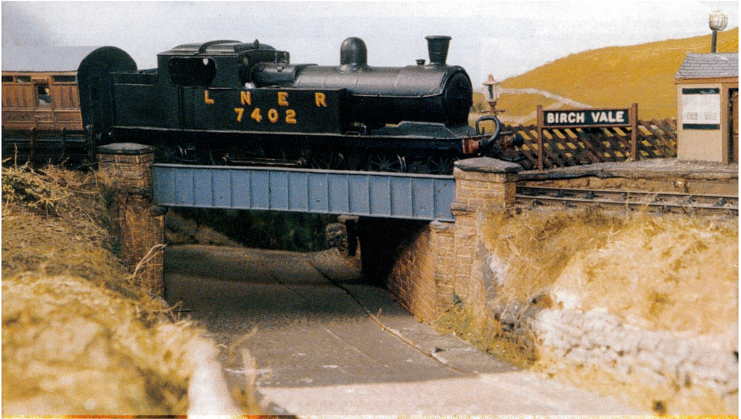
As a schoolboy I 'footplated' 7402 from Hyde Junction to Macclesfield and back, some 50-60 miles. The body is Slater's 'Plastikard' and was my very first attempt at scratch-building! The chassis was my first attempt in 18.83mm gauge and later was used to prove that I could cope with S4 standards. Much nostalgia for me in this picture. It's the third chimney and still not quite right!
